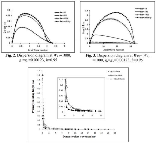
**Fig. 3.** The Effect of Liquid Viscosity on the primary break up of spray at  $We_i = We_s = 1000$ ,  $g_i = g_o = 0.00123$ , h = 0.95
