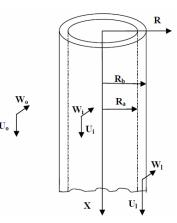
Fig. 1. Annular swirling viscous liquid sheet subject to swirling airstreams
