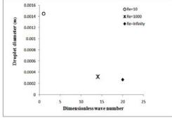
Fig. 4. The Effect of Liquid Viscosity on Droplet diameter at  $We_i = We_s = 1000$ ,  $g_i = g_o = 0.00123$ , h = 0.95
