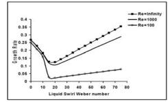
Fig. 7. Liquid Swirl Weber number Vs Growth Rate at  $We_l=1000$ ,  $g_i=g_o=0.00123$ , h=0.95
