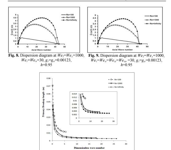
**Fig. 10.** The Effect of Liquid Viscosity on the primary break up of spray at  $We_i = We_s = 1000$ ,  $We_i = We_o = We_{si} = We_{so} = 30$ ,  $g_i = g_o = 0.00123$ , h = 0.95
