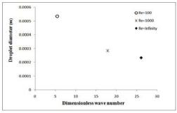
**Fig. 12.** The Effect of Liquid Viscosity on Droplet diameter at  $We_i = We_s = 1000$ ,  $We_i$  $= We_o = We_{si} = We_{so} = 30$ ,  $g_i = g_o = 0.00123$ ,
